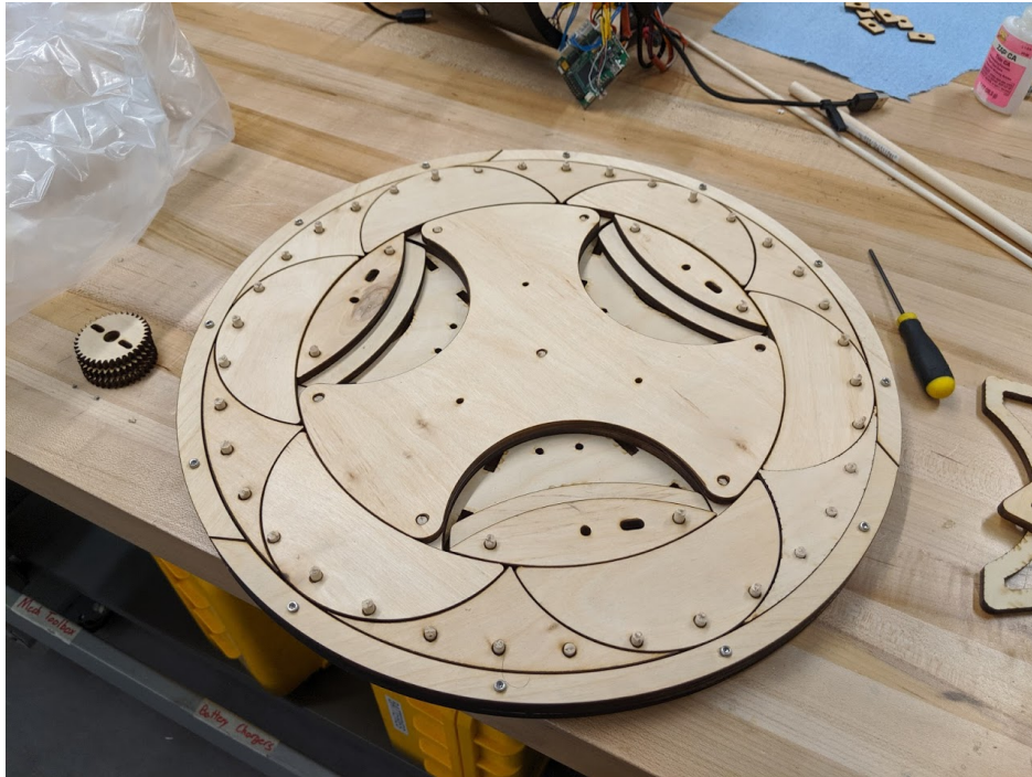
Figure 4: Test fit of laser cut parts with alignment pegs
