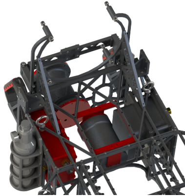
Figure 11: Enclosures, Plates, and Mounting at the Fore End
