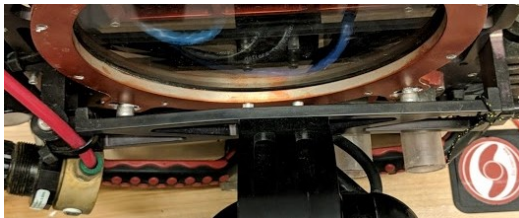
(a) Plastic Deformation on Castor
