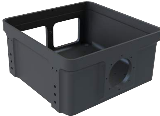
Figure 5: Pollux's UHPV's hull. Opening on the right for the forecam, holes along the side for mounting draw latches and to the frame.
