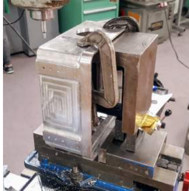
Figure 13: Fixturing the hull to add the fore camera's mounting holes.
